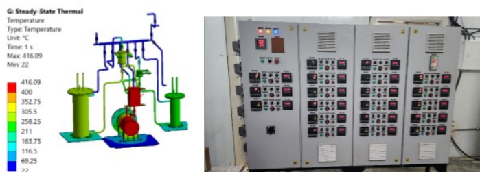
Figure A.2.9: Steady-state thermal analysis of Tin-Lithium Loop (Left). PID based temperature controller is energized and ready for integration with Tin-Lithium Loop (Right).
