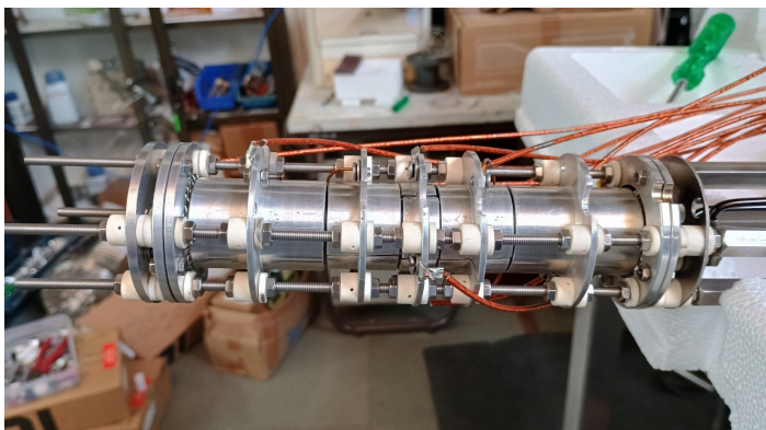
Figure A.3.7: Linear cylindrical Penning – Malmberg Trap made up of five concentric cylindrical ring electrodes, grids and filament.
