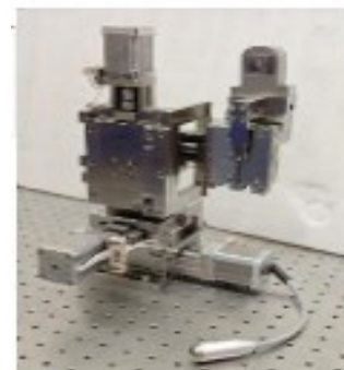
Figure B.1.24: A 40-channel prototype fiber bundle & magnetic field compatible motor (0.3T).
