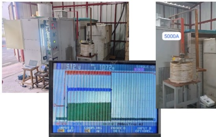
Figure B.1.21: 5kA/500V Thyristor Converter Test Setup and Results at Aditya-U extended Shed.
