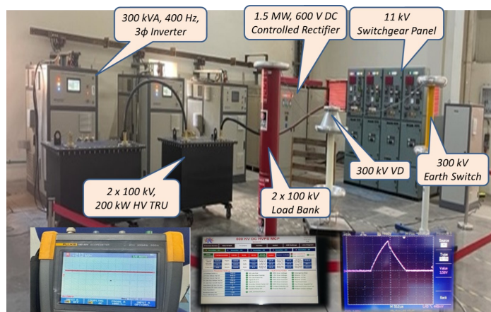
Figure A.6.2: Development of 300kV, 2A DC power supply.
