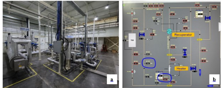
Figure A.2.20: a) Photograph of EHCL system b) Hot testing results of EHCL at 300°C, 80 bar conditions.
