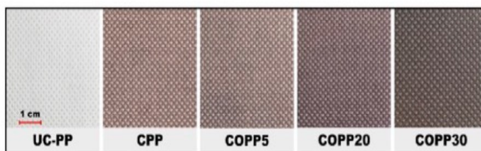
Figure A.4.2: Coated and un-coated fabric: Uncoated polypropylene (UC-PP), Copper coated polypropylene (CPP), Copper oxide at 5 % Oxygen partial pressure (COPP5), Copper oxide at 20% oxygen partial pressure (COPP20), copper oxide at 30 % Oxygen partial pressure (COPP30).
