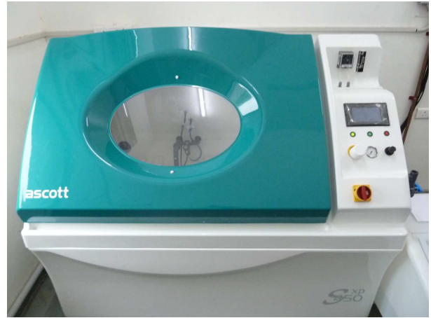
Fig. 2: Salt Spray Chamber supplied by Ascott Analytical Equipment Ltd.
