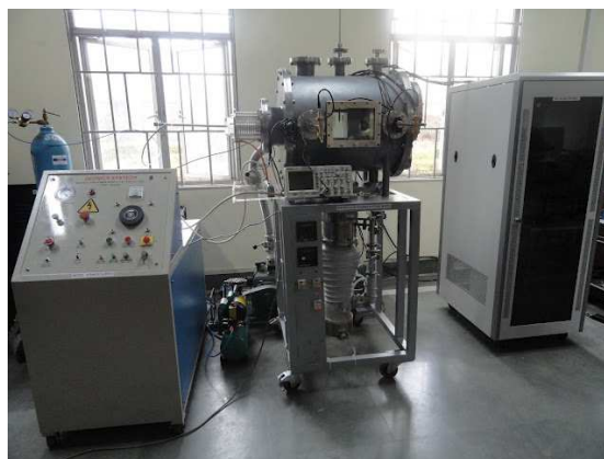
Fig.1: Washer gun plasma system installed at Delhi University.
