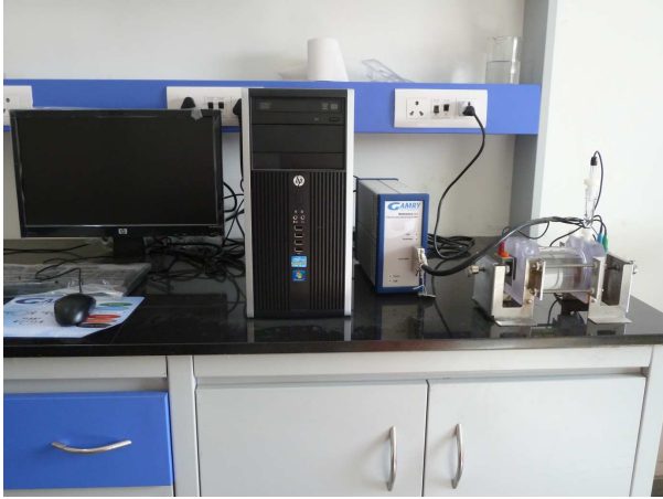
Fig. 1: Potentiodynamic set-up supplied by M/s Gamry Instruments, USA.
