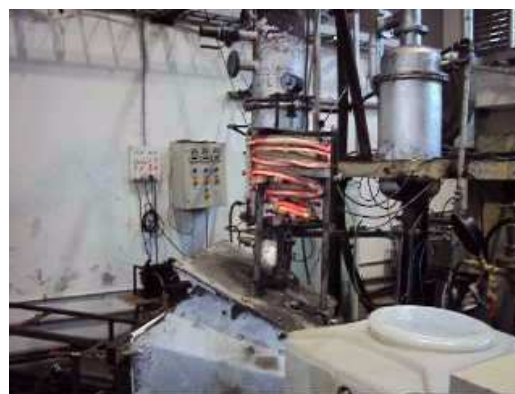
Fig. 1: Image of the plasma gasification system with the arrangement to feed Tank Sludge
