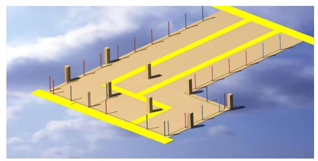
Layout of earth strips inside the lab. Two strips for single-phase (green) and three-phase (red) are there in the layout
