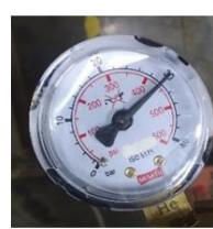
Hot Helium Leak Test (Temp \sim 140 deg C, Pressure 30 bar, achieved leak rate in the range of 10^{-9} mbarl/s)
