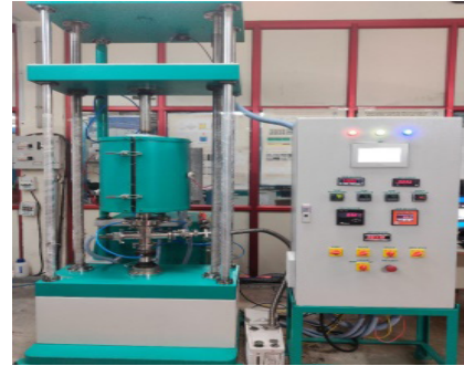
Figure A.4.22: Experimental facility for Pebble bed thermos-mechanical experiments.
