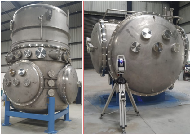
Figure B.2.2: BSC and HAM (1:1) size prototype chambers (1 each) recently delivered at RRCAT.
