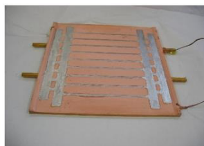
Surface activation by Silver Paint- ready for electrodeposition
