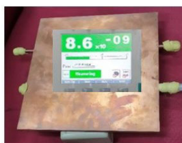
Electro-deposited plate- He leak tightness in the range of 10^{-9} mbarl/s
