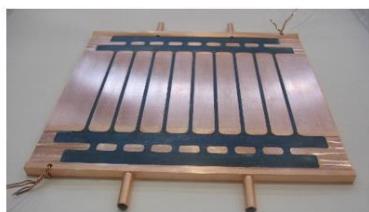
Plate with cooling channels filled with 'WAX'
