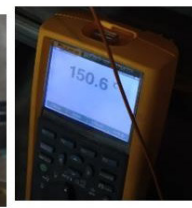
Hot Helium Leak Test (Temp \sim 140 deg C, Pressure 30 bar, achieved leak rate in the range of 10^{-9} mbarl/s)
