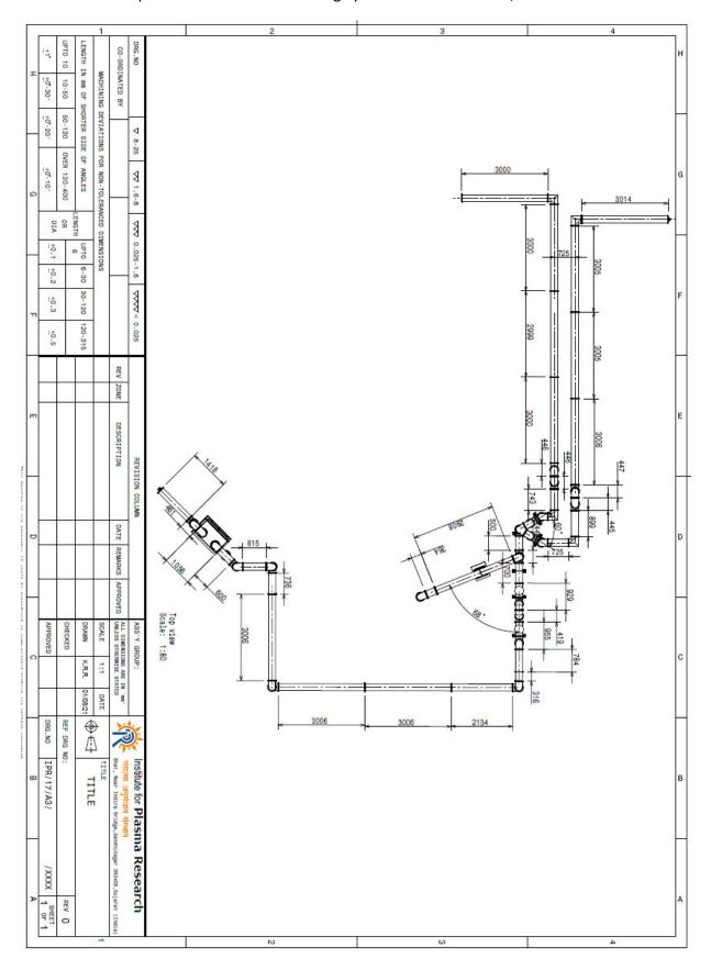
Annexure-IV: Side view of Tx-line & matching system inside SST1 Hall/ICRH Area
