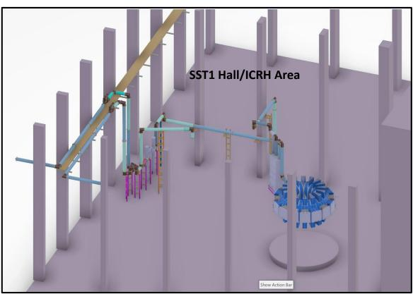
Annexure-II: Overview of Tx-line & matching system layout inside SST1 Hall/ICRH Area
