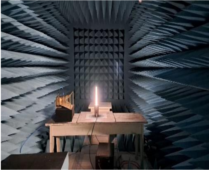
Fig. Radiation Pattern measurement at Anechoic chamber
