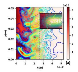
**Figure :** Superposition of (a) Ar<sup>+</sup>, (b) Ne<sup>+</sup>, and (c) N<sup>+</sup> (contour lines) with plasma density ("Reds," colormap).  $\frac{1}{5}$ The region on the left side of the vertical dotted line is edge and on the right side of it is SOL.
