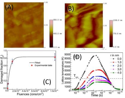
Figure Caption: (a) Pristine & (b) irradiated 5x5  $\mu$ m AFM image (c) Variation of damaged fraction as a function of Au fluence for (012) diffracted peak (d) Variation of lattice temperature as a function of time for different radii around the ion track for Se =17.19 keV/nm and Sn =5.5 ×10<sup>3</sup> keV/nm using u-TS model.
