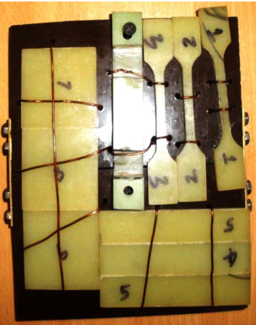
Fixing assembly of GFRP insulation samples in Reactor
