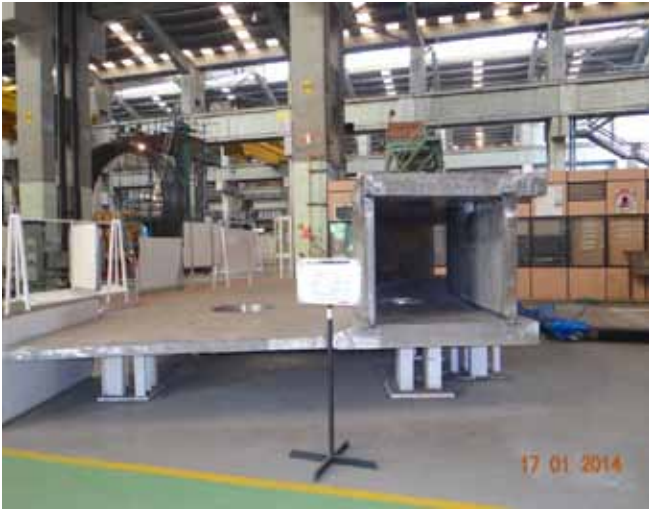
Figure B.2.1 Cryostat Base Section Mockup
