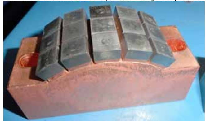
Figure A.2.2.3 Curved Tungsten Macro-Brush brazed with CuCrZr substrate
