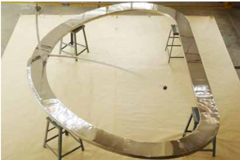
Figure A.2.1.1 Prototype magnet (8-turn single layer) wound with indigenous CIC superconductors of 30kA rating
