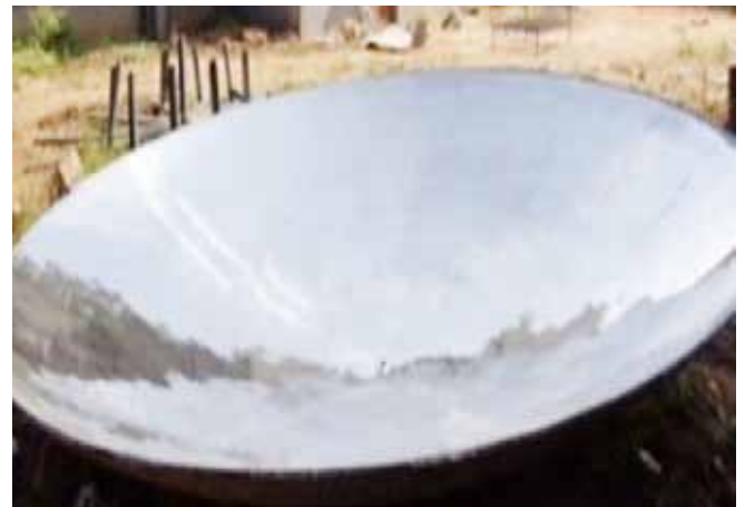
Figure A.2.7.3.1 Manufacturing of the INTF Vacuum vessel at vendor's site.
