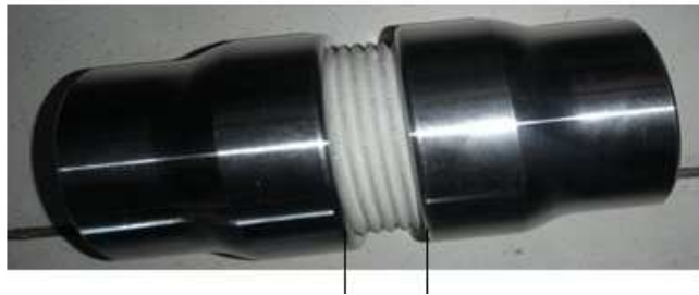
Filament winding section from 125 mm ID to 143 mm OD of 15 mm section
