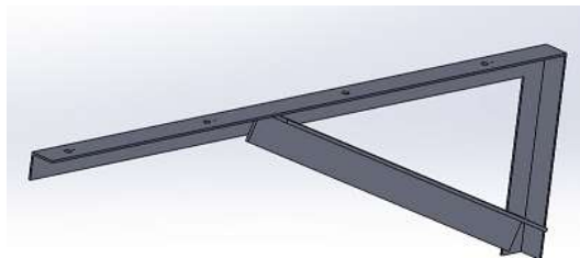
Figure-4 (Wall Support)
