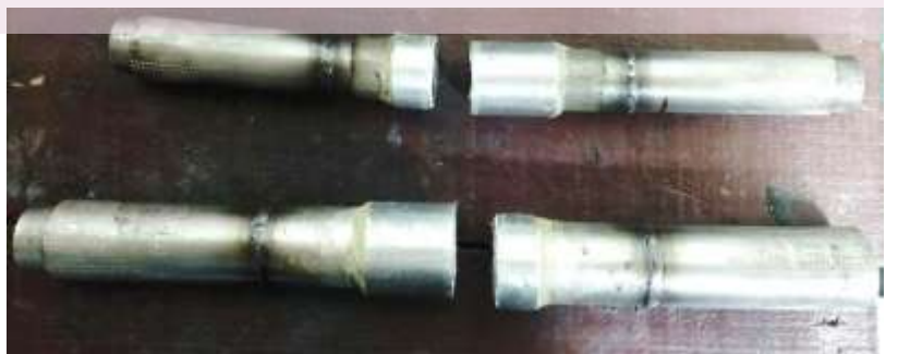
(L) SS-Al bi-metallic joints (R) SS-Al bi-metallic joint after tensile pull test
