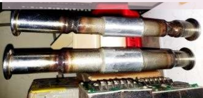
(L) SS-Al bi-metallic joints (R) SS-Al bi-metallic joint after tensile pull test
