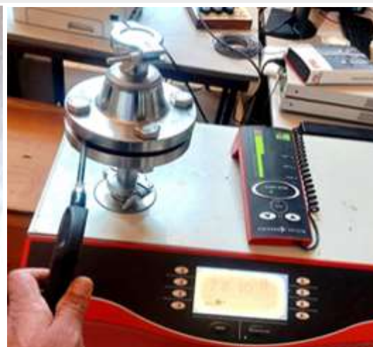
Helium leak test
