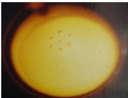
Single hexagonal structure of water droplets formed after adjusting the oppositely charged background.
