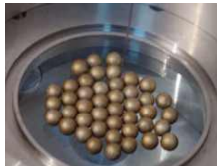
Coulomb crystals created using centimeter sized spherical objects.
