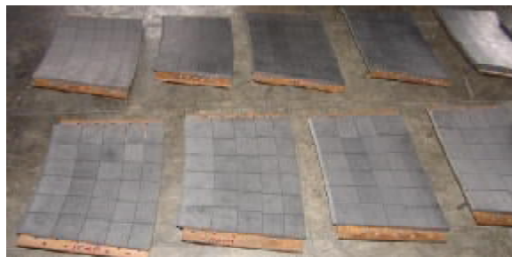
Graphite tile assembly of the outer passive stabilizer.
