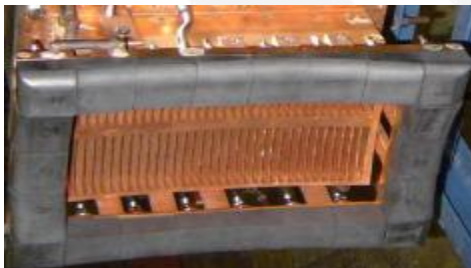
Photograph of the LHCD grill antenna
