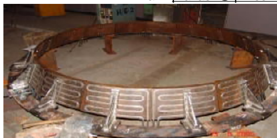
Module Assembly of the outer divertor.
